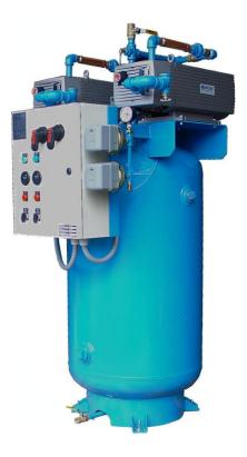
and alarm functions will remain energized while any vacuum pump in the system remains electrically on-line. Field adjustable control switches are pre-set to operate the lead vacuum pump between 19" Hg and 22" Hg. The lag vacuum pump will automatically start at 18" Hg if the lead vacuum pump fails to operate.
